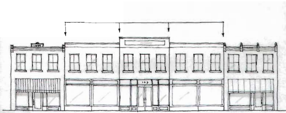
Large new buildings should be designed with vertical divisions to be consistent with traditional historic building widths.
