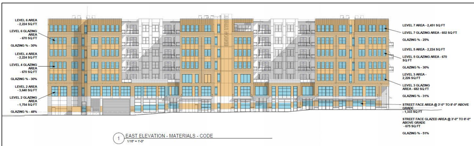
Diagram detailing the glazing on the front building elevation.
