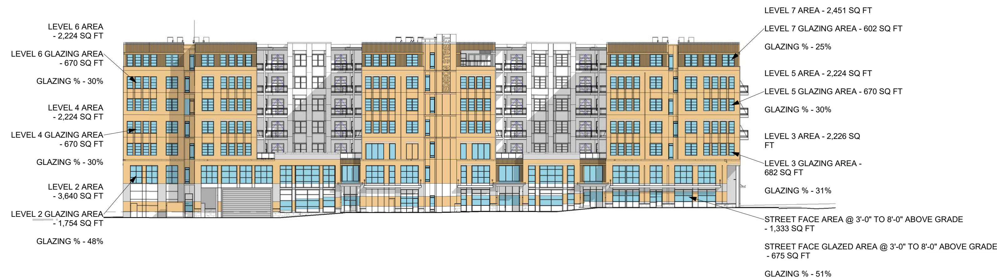
2 EAST ELEVATION - MATERIALS 1" = 30'-0"
