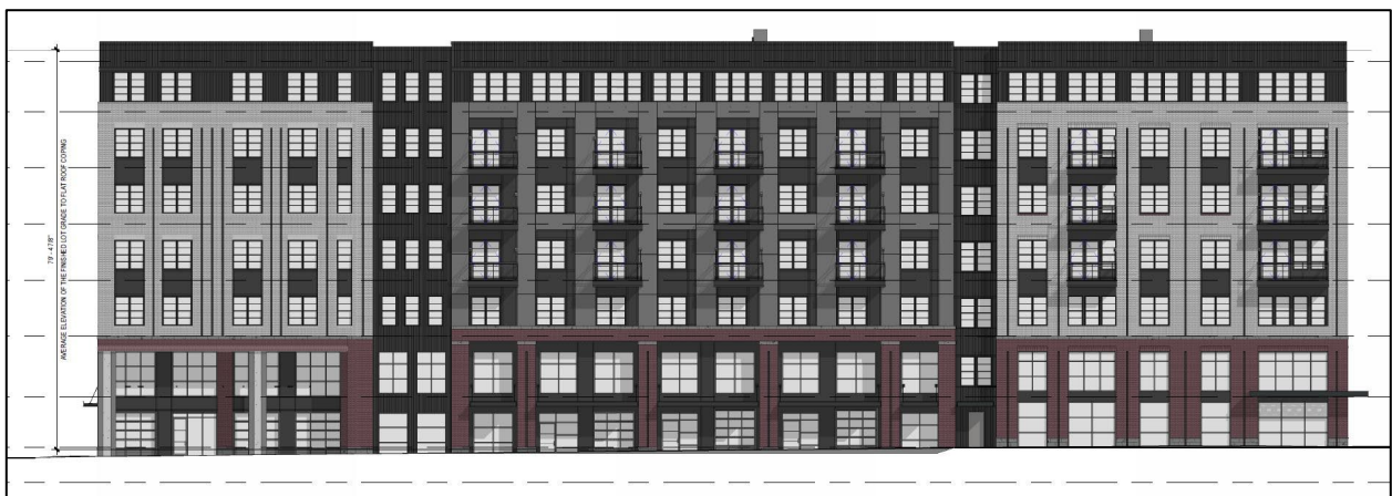
Northern elevation (midblock walkway) – average height of 79'6"
