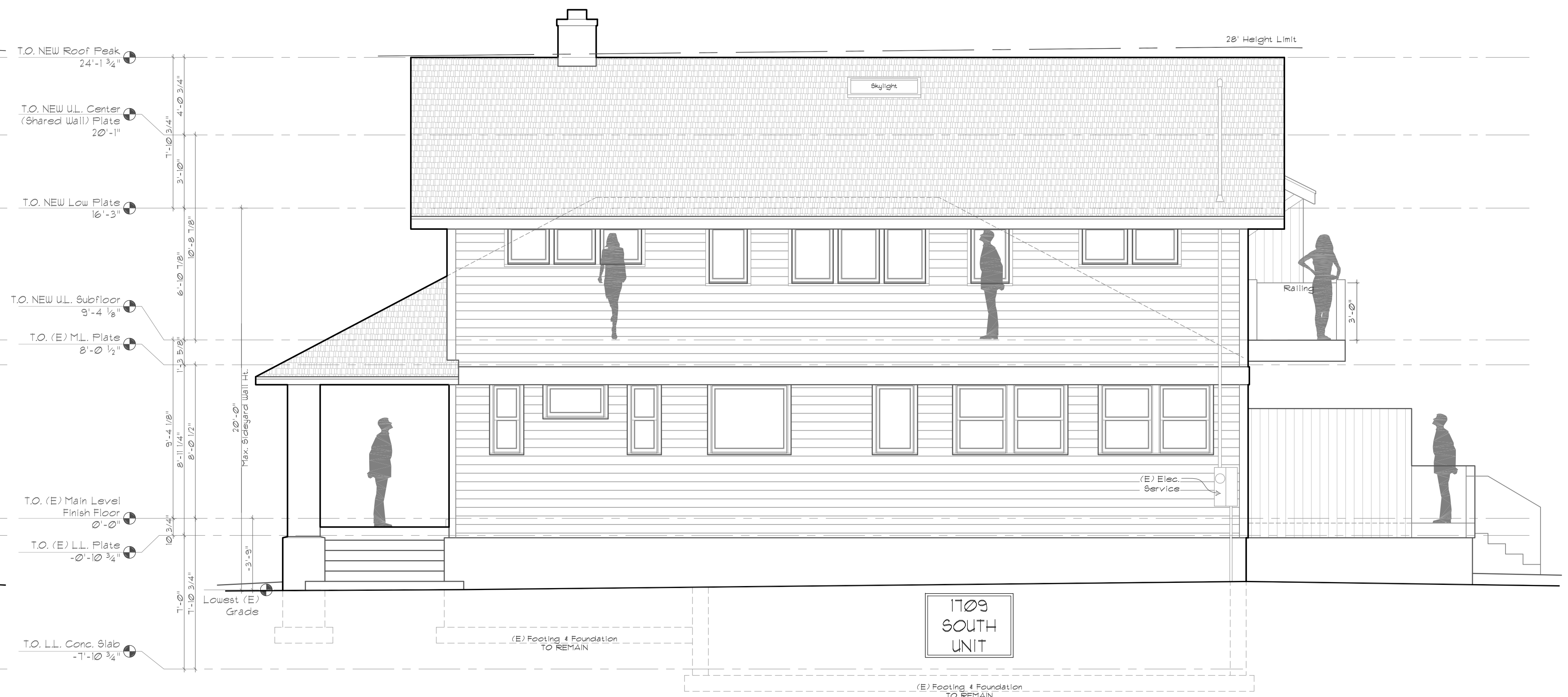
4 WINDSOR DUPLEX - PROPOSED EXTERIOR ELEVATION- SOUTH SCALE: 1/4"=1'-0"
