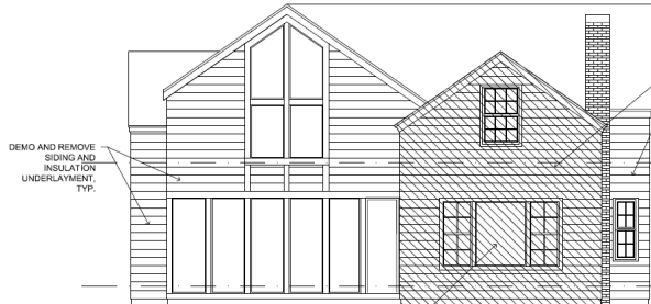
WEST ELEVATION - EXISTING SCALE: 1/4" = 1'-0"
