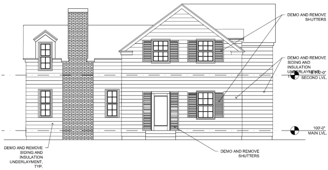
SOUTH ELEVATION - EXISTING SCALE: 1/4" = 1'-0"
