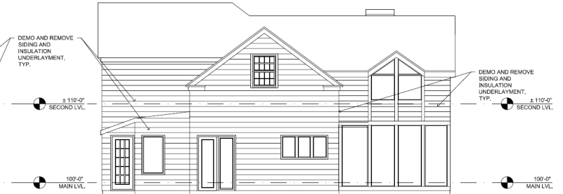
NORTH ELEVATION - EXISTING SCALE: 1/4" = 1'-0"
