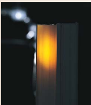
Light penetration of competitor's vinyl material
